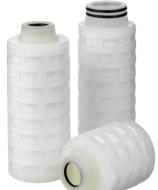
The construction utilises thermal welding techniques to bond all the components, therefore eliminating adhesives, minimising extractables and optimising cartridge integrity.
